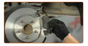
Replacement: brake pads – FORD Transit Connect V408 Van. Tip from AUTODOC:
