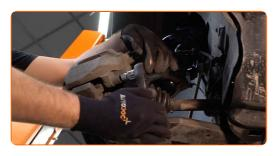
Remove the brake caliper.
