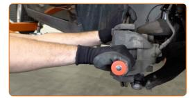
Detach the brake caliper retaining spring. Use a crowbar.
