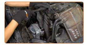
Tighten the upper fastener of the engine mount. Use a drive socket #16. Use a torque wrench. Tighten it to 57 Nm torque.
