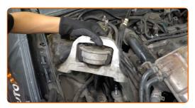
Replacement: engine mounts – FORD TRANSIT CONNECT (P65\_, P70\_, P80\_).
