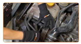
Release the coolant reservoir retainers. Use a flat screwdriver.
