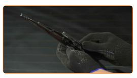
Remove the blade from the wiper arm.
