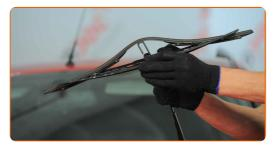
Remove the blade from the wiper arm.
