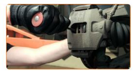
Remove the brake caliper.
