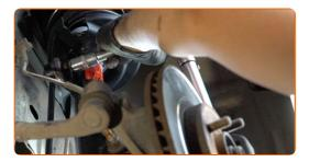
Tighten the fastener connecting the stabilizer link to the stabilizer bar. Use a drive socket #15. Use a torque wrench. Tighten it to 48 Nm torque.
