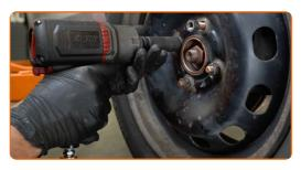
Lower the car and working in a cross order, tighten the wheel bolts. Use wheel impact socket #19. Use a torque wrench. Tighten it to 110 nm torque.
