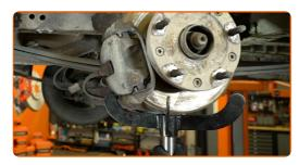
Tighten the lower fastener of the shock absorber. Use a 15 mm combination spanner. Use an 18 mm socket. Use a torque wrench. Tightening torque: 80 N·m.
