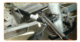
Tighten the top fastener of the shock absorber. Use an 18 mm combination spanner. Use a 21 mm socket. Use a torque wrench. Tightening torque: 180 N·m.
