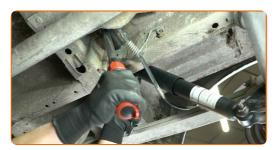
Remove the support from under the axle beam.
