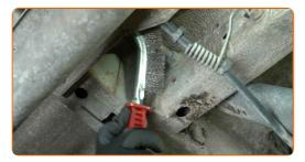
Prop up the rear axle beam. If the car has been raised on a lift, use a hydraulic transmission jack.
