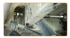
Unscrew the lower fastener of the shock absorber. Use an 18 mm combination spanner. Use a 15 mm socket. Use a ratchet wrench.
