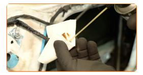
Attach the connector to the speaker.
