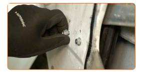
Remove the window regulator mechanism.
