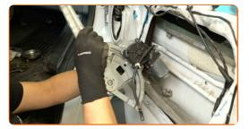
Install a new window regulator mechanism.
