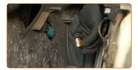
Unscrew the fasteners of the speaker. Use a Phillips screwdriver.
