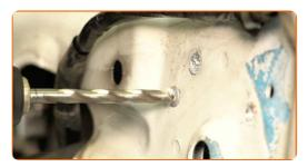
Unscrew the window guide rail fastener. Use an 8 mm socket. Use a ratchet wrench.
