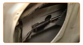
Install the fastening bolt of the window guide rail.
