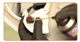
Treat the connector of the power window switch. Use an electronic spray.
