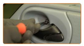
Tighten the door card fasteners. Use a Phillips screwdriver.
