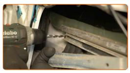
Drill out the rivets connecting the window regulator mechanism to the door. Use a drill. Use a drill bit set.
