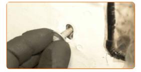
Tighten the window guide rail fastener. Use an 8 mm socket. Use a torque wrench. Tightening torque: 6 N·m.
