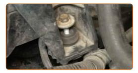
Screw in the fasteners of the air filter housing. Use a 10 mm socket. Use a ratchet wrench.
