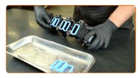
Remove the paper towels from the intake manifold openings.
