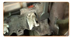
Remove the intake manifold gaskets.
