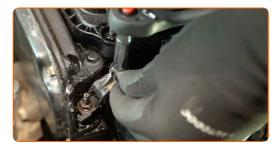
Detach the fuel pressure sensor connector.
