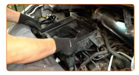
67 Secure the rubber hoses on the air filter housing.
