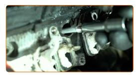
Tighten the glow plugs. Use a 10 mm glow plug socket. Use a torque wrench. Tightening torque: 13 N·m.
