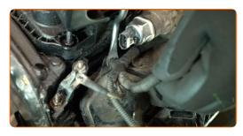
Clean the fasteners of the oil dipstick tube bracket. Use a wire brush. Use WD-40 spray.
