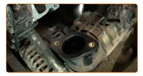
Install the intake manifold.
