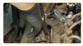
Unscrew the intake manifold fasteners. Use a 10 mm socket. Use a ratchet wrench.
