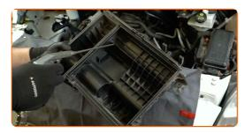
66 Install the air filter housing.
