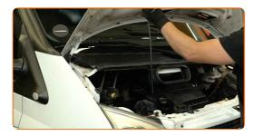
Use a fender protection cover to avoid damaging the paintwork and plastic parts of the car.
