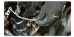
Attach the glow plugs power cable terminal and screw on the nut that secures it. Use an 8 mm socket. Use a ratchet wrench.
