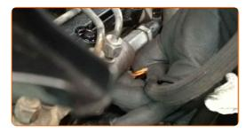
Attach the fuel pressure sensor connector.
