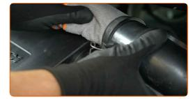
Connect the air intake hose to the air filter housing.
