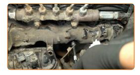
Remove the intake manifold.
