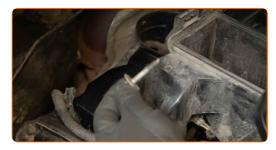
Detach the rubber hoses from the air filter housing.
