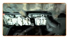
Screw on the power terminal nuts.
