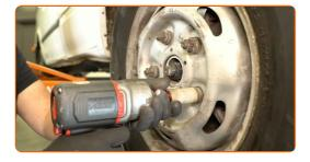
Lower the car and tighten the wheel nuts in a criss-cross pattern. Use a 21 mm wheel impact socket. Use a torque wrench. Tightening torque: 200 N·m.
