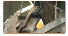
Install and screw in the fastening bolt.
