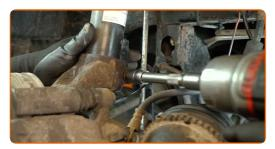
Remove the fastening bolt.
