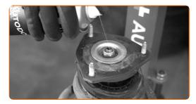
Unscrew the strut piston rod nut. Use an 18 mm strut nut socket. Use an H6 hex extension bar. Use a ratchet wrench.
