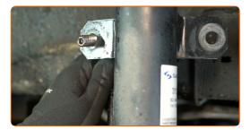
Unscrew the axle nut. Use a 36 mm socket. Use a ratchet wrench.
