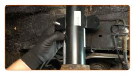
Install the ABS sensor cable bracket and screw on the fastening nut.
