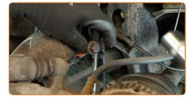
Disconnect the steering knuckle from the suspension strut. Use a rubber mallet. Use a transmission jack or one more vehicle jack.
