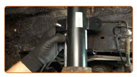
Install the ABS sensor cable bracket and screw on the fastening nut.
