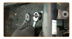
Disconnect the anti-roll bar link from the suspension strut.
