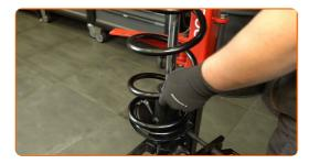
Install a dust boot, bump stop, and mount bearing.
