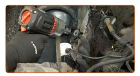
Unscrew the fastener connecting the anti-roll bar link to the suspension strut. Use a 19 mm combination spanner. Use an H5 hex bit. Use a ratchet wrench.
