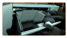
Fold back the insulation that covers the strut mount fasteners.
