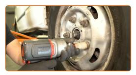
Lower the car and tighten the wheel nuts in a criss-cross pattern. Use a 21 mm wheel impact socket. Use a torque wrench. Tightening torque: 200 N·m.
