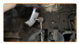
Clean the splines of the CV axle joint. Use a wire brush. Use an all-purpose cleaning spray.
