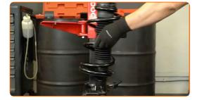
Install the strut assembly into the wheel arch.
