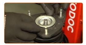
Install and tighten the strut piston rod nut. Use an 18 mm strut nut socket. Use an H6 hex extension bar. Use a torque wrench. Tightening torque: 70 N·m.
