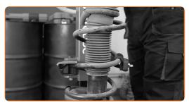
Clean the top part of the strut piston rod. Use a wire brush. Use WD-40 spray.
