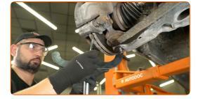
Disconnect the ball joint from the suspension arm. Use a ball joint separator. Use a mounting lever.
