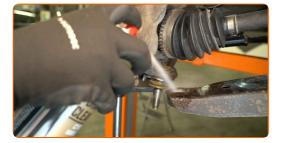
Attach the ball joint to the suspension arm and screw on the fastening nut. Use a mounting lever.
