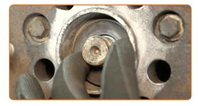
Screw on the axle nut. Use a 36 mm socket. Use a ratchet wrench.
