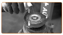
Unscrew the strut piston rod nut. Use an 18 mm strut nut socket. Use an H6 hex extension bar. Use a ratchet wrench.
