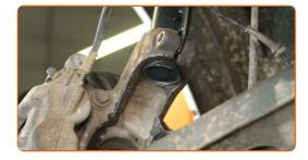
70 Install and screw in the fastening bolt.
