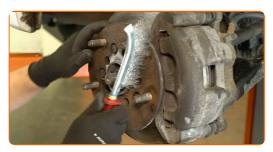
Treat the wheel hub surface that contacts the wheel rim. Use ceramic grease.
