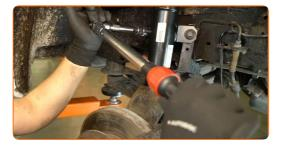
77 Tighten the fastener of the ABS sensor cable bracket. Use an 18 mm socket. Use a torque wrench. Tightening torque: 45 N·m.
