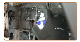
Loosen the nut fitting connecting the brake pipe to the brake hose. Use an 11 mm flare nut wrench. Use a 17 mm combination spanner.
