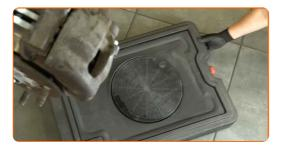
Clean the areas where the brake hose is connected to the brake caliper and to the brake pipe. Use a wire brush. Use WD-40 spray.
