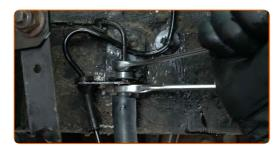
Tighten the brake hose nut fitting on the brake caliper. Use an 11 mm flare nut wrench. Use an 11 mm flare nut socket. Use a torque wrench. Tightening torque: 15 N·m.
