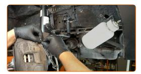
Loosen the brake bleeder screw. Use an 11 mm combination spanner.
