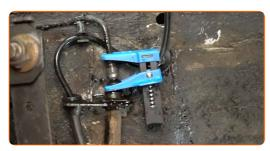
Detach the brake hose from the brake caliper. Use an 11 mm flare nut wrench.
