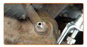
Clean the bleeder screw. Use a wire brush. Use a brake cleaner.
