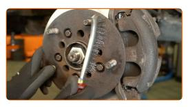
Treat the wheel hub surface that contacts the wheel rim. Use ceramic grease.
