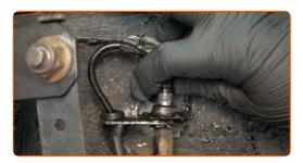
Block off the brake pipe. Use a fluid line stopper.
