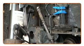
Clean the brake hose mounting seat on the brake pipe. Use a wire brush. Use a brake cleaner.
