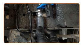
Install the brake hose retaining clip. Use a hammer.
