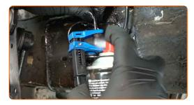
Clean the area where the brake hose connects to the caliper. Use a wire brush. Use a brake cleaner.
