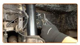
Clean the mounting seats of the anti-roll bar link on one side of the axle. Use a wire brush. Use an all-purpose cleaning spray.
