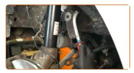
Install a new anti-roll bar link and its fasteners.
