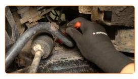
Unscrew the fasteners of the anti-roll bar bush bracket. Use a 10 mm socket. Use a ratchet wrench.
