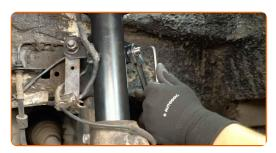
Clean the bracket fasteners of one of the anti-roll bar bushes. Use a wire brush. Use WD-40 spray.
