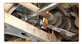
Tighten the fastener connecting the anti-roll bar link to the suspension strut. Use a 20 mm combination spanner. Use a 17 mm socket. Use a torque wrench. Tightening torque: 55 N·m.
