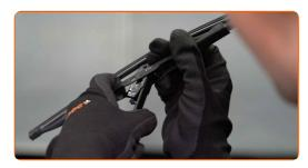
Remove the blade from the wiper arm.
