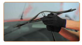
Remove the blade from the wiper arm.
