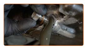
Replacement: engine oil and filter – FORD Tourneo Custom V362 Minibus (F3).
