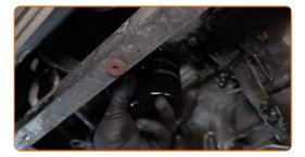
Tighten the oil filter. Remember to observe the recommended tightening torque. Use the 76-14F socket. Use a torque wrench. Tighten it to 24 Nm torque.
