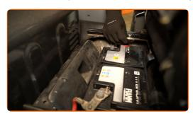
Unscrew the positive battery terminal fastener. Use a 10 mm socket. Use a ratchet wrench.
