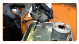
Install and tighten the cap of the fuel filter housing. Use Torx T15. Use a ratchet wrench.
