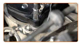
Attach the fuel pressure sensor connector.
