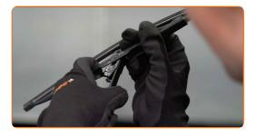
Remove the blade from the wiper arm.
