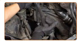
Unscrew the fasteners that connect the engine mount to the car body. Use a drive socket #16. Use a ratchet wrench.
