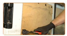
Remove the number plate light. Use long nose pliers.
