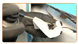
Attach the connector to a new number plate light.
