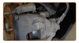
Install the brake caliper retaining spring.
