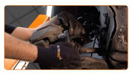
Remove the brake caliper.
