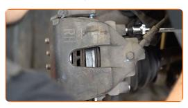
Install the dust boot caps of the brake caliper guide pins.
