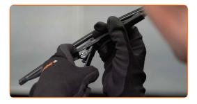
A Remove the blade from the wiper arm.
