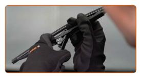
Remove the blade from the wiper arm.
