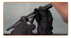
Remove the blade from the wiper arm.
