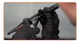
Remove the blade from the wiper arm.
