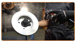
19 Install the brake disc.
