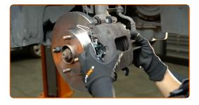
24 Install the brake caliper retaining spring.
