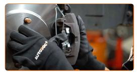
Tighten the brake caliper fasteners. Use HEX No.H7. Use a torque wrench. Tighten it to 28 Nm torque.
