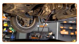
Replacement: engine oil and filter – FORD Sierra Mk2 Hatchback (GBC, GBG). Tip:
