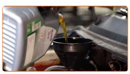
Replacement: engine oil and filter – FORD Sierra Mk2 Hatchback (GBC, GBG).
