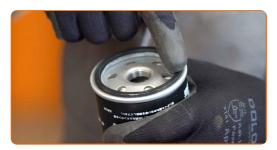
Screw the new filter into its place. Use the 76-30F socket. Use a torque wrench. Tighten it to 18 nm torque.
