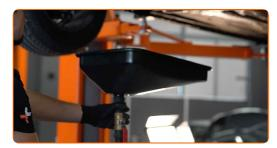
Unscrew the drain plug. Use a drive socket #13. Use a ratchet wrench.
