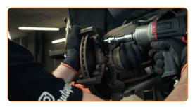
Remove the caliper bracket.
