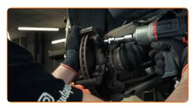
Remove the caliper bracket.
