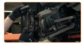
16 Remove the brake disc.
