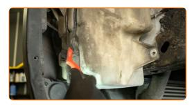
Detach the connector from the windscreen washer pump. Use a mounting lever.
