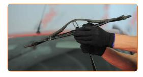
Remove the blade from the wiper arm.
