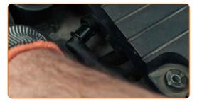
Remove the air intake pipe.
