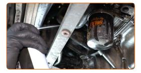
Unscrew the oil filter. Use the 76-14F socket. Use a ratchet wrench.
