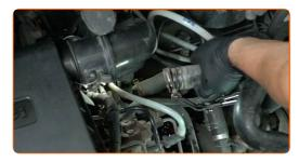
Clean the fasteners of the thermostat housing cover. Use a wire brush. Use an all-purpose cleaning spray.
