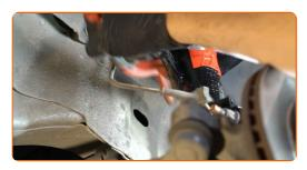
Install a new rod, tighten the fasteners. Use a combination spanner #15. Use HEX No.H5. Use a ratchet wrench.
