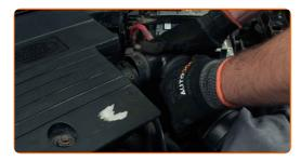
Detach the air intake hose clamp. Use clic-R collar pliers.
