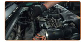
Screw new spark plugs and tighten them. Use the spark plug socket #16. Use a torque wrench. Tighten it to 15 nm torque.
