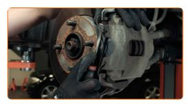
11 Remove the brake caliper.
