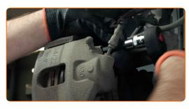
Detach the brake caliper retaining spring. Use a crowbar.
