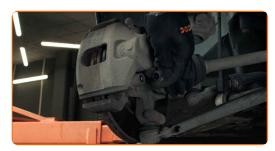
9 Unscrew the brake caliper fastening. Use HEX No.H7. Use a ratchet wrench.
