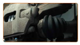
20 Install the brake caliper retaining spring.
