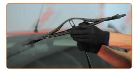
Remove the blade from the wiper arm.
