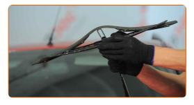
Remove the blade from the wiper arm.
