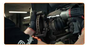
Remove the caliper bracket.
