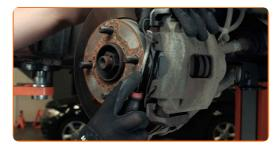
11 Remove the brake caliper.
