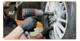
Lower the car and working in a cross order, tighten the wheel bolts. Use wheel impact socket #19. Use a torque wrench. Tighten it to 95 Nm torque.
