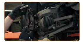
16 Remove the brake disc.
