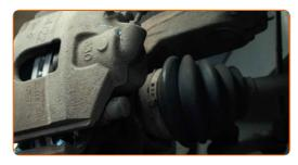
Install the brake caliper retaining spring.
