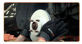
20 Install the brake caliper bracket.
