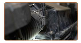
Remove the air intake pipe. Use a crowbar.
