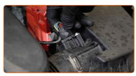
Detach the air intake hose clamp. Use a drive socket #7. Use a ratchet wrench.
