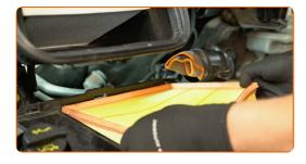
Unscrew the fasteners of the air filter housing. Use a 10 mm socket. Use a ratchet wrench.
