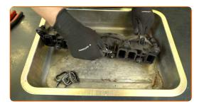
Clean the intake manifold. Use a nylon brush. Use an all-purpose cleaning spray.
