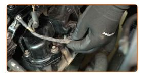
Attach the glow plugs power cable terminal and screw on the nut that secures it. Use an 8 mm socket. Use a ratchet wrench.
