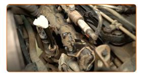
Plug the intake manifold openings with paper towels to prevent dust and dirt from getting into the system.
