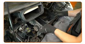
Clean the connectors of the fuel pressure, MAP and camshaft position sensors. Use an all-purpose cleaning spray.
