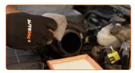
12 Install the air duct housing.
