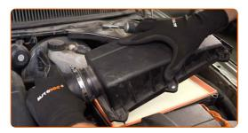
Reinstall the air filter cover. Fasten it.
