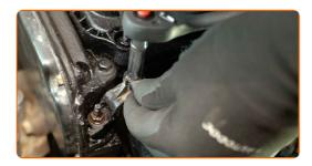
Detach the fuel pressure sensor connector.
