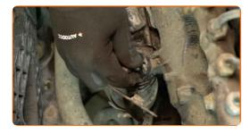
Detach the air intake hose from the intake manifold.
