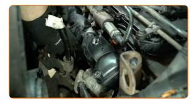
Tighten the intake manifold fasteners. Use a 10 mm socket. Use a torque wrench. Tightening torque: 25 N·m.
