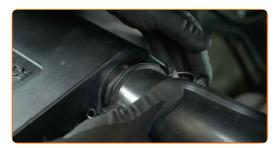
75 Snap the air intake hose clips into place.
