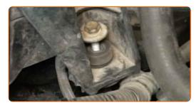
Screw in the fasteners of the air filter housing. Use a 10 mm socket. Use a ratchet wrench.
