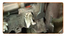
Remove the intake manifold gaskets.
