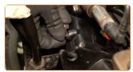
Screw in the fasteners of the oil dipstick tube bracket. Use an 8 mm socket. Use a ratchet wrench.
