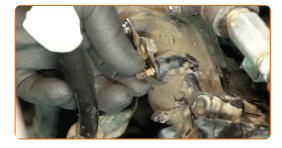
Clean the intake manifold fasteners. Use a wire brush. Use WD-40 spray.
