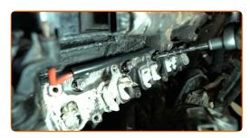
Clean the intake manifold mounting seat. Use a gasket scraper. Use an all-purpose cleaning spray.
