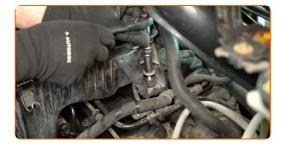
70 Install the filter element.
