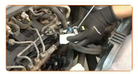
Install and secure the wiring harness.
