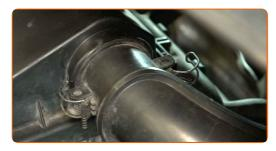
Disconnect the air intake hose from the air filter housing.
