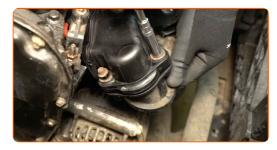
Screw in the fasteners that connect the air intake hose to the intake manifold. Use a 13 mm socket. Use an 8 mm socket. Use a ratchet wrench. Use a U-joint socket extension.
