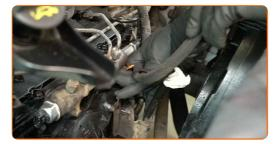
Attach the camshaft position sensor connector.
