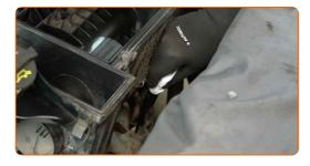
14 Remove the air filter housing.
