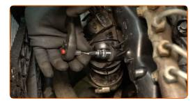
Install the fasteners of the oil dipstick tube bracket.
